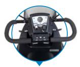
All operational controls including lights, horn and battery display are conveniently located in the center of the one-hand operation Delta handlebar
