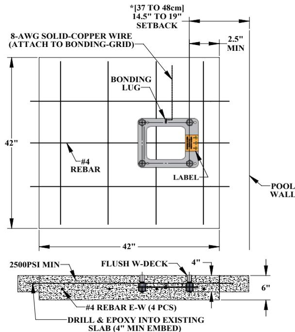
\*SETBACK DIMENSIONS ARE FOR **FLAT DECK** APPLICATIONS. FOR SLOPED DECKS OR OTHER FEATURES, CONTACT AQUA CREEK BEFORE INSTALLATION.
