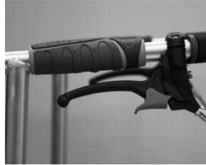
then the brake lever. Make sure the locking mechanism is fixed in position. Make sure the Velped does not move.
