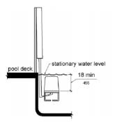
Figure 1009.2.8 Pool Lift Submerged Depth
