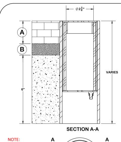
**ANCHOR DESIGNED FOR COMPATIBILITY** WITH MOTION TREK BP 350 OR SIMILAR LIFT ONLY.
