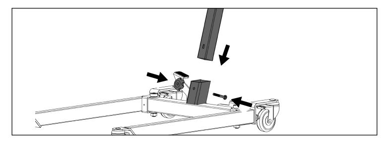
Step 4: Remove the plastic knob and bolt on the boom. Do not remove the plastic U shaped washer or the bushing inside the hole of the boom, reinsert and align the holes of the plastic washer and bushing if needed.
