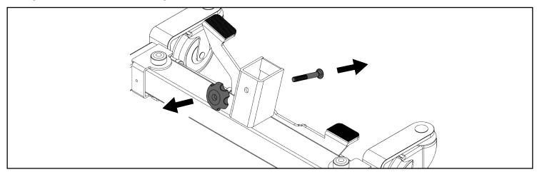
Step 3: Insert the mast into the base bracket, align the holes on the bracket with hole on the mast. Reinsert the bolt and the plastic knob. Tighten the plastic knob.
