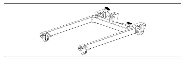
Step 2: Remove the plastic knob and bolt from the base bracket.
