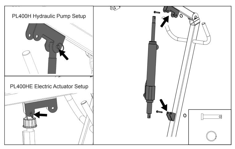
Install the spreader bar to the bracket at the end of the boom, and secure spreader using a pin and retaining ring as follows.
