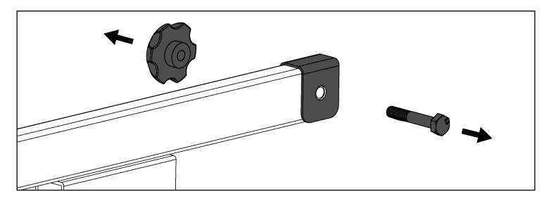
Step 4: Insert the boom with the plastic washer as follows into the bracket at the top of the mast. Resert the bolt and plastic knob, and tighten the plastic knob.
