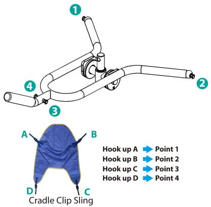
BEFORE LIFTING THE PATIENT, PULL ON **EACH** SLING LOOPS TO ENSURE THE LOOP IS HOOKED ONTO THE SPREADER BAR PROPERLY
