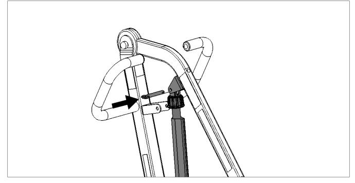
**Step 10**: Insert the spreader bar into the tube on the boom as follows. Align the holes and secure the spreader bar using a pin and retainer ring.
