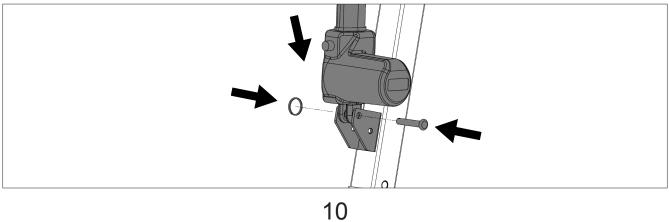
**Step 9**: Install the upper end of actuator to the boom by reinsert the quick release pin to secure it.
