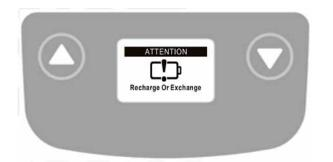
If the battery is critically low, the LCD Display Panel will show the sign on the left either when the emergency stop button is released or when a button on the LCD Display Panel is pressed.
