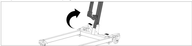
Step 5: Insert the pin to secure the mast.
