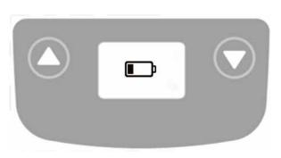
If the battery needs to be charged, the LCD Display Panel will show a blinking low battery sign shown on the left either when the emergency stop button is released or when a button on the LCD Display Panel is pressed.
