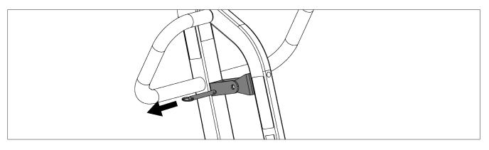
Step 7: Remove lower actuator pin on the mast.
