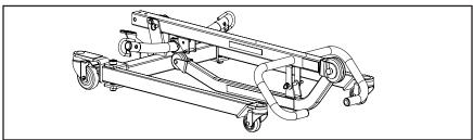
**Step 2**: Secure the stand to the mast. Hold the nut on its side with two fingers. Align the nut and the hole on the stand bracket with the lower hole on the mast. Make sure the tab on the stand bracket sit in the top hole on the mast, and insert the screw to the nut as follows. Use the EZ-Tools to tighten the screws.
