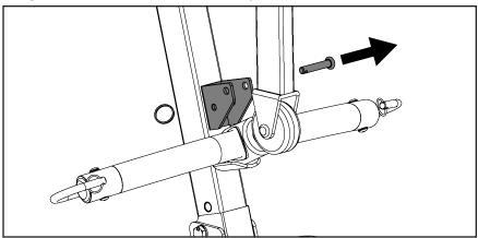
Step 8: Move the boom out of the way, and install the lower end of the actuator as follows
