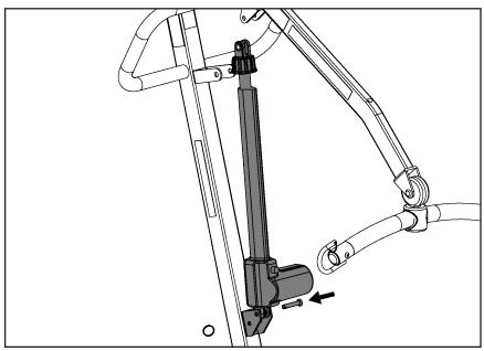
**Step 9**: Install the upper end of actuator and reinsert the quick release pin to secure it.
