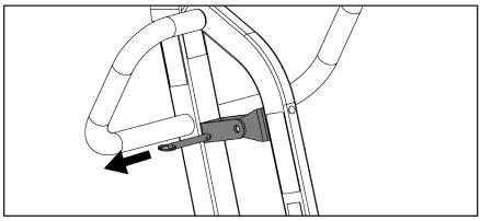
**Step 7**: Remove lower actuator pin
