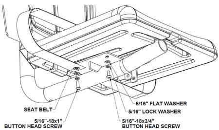
Note: When attaching the seat belt use 5/16"-18 x 1" as shown below.
