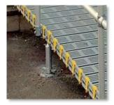
Note: Be sure stands are installed on the same link on each side.
