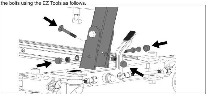
**Step 5**: Remove the plastic caps, then all the bolt, nut and washers on the boom. Tighten the bolt and nut using the EZ Tools as follows.
