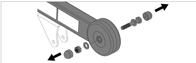
**Step 6**: Secure the boom to the mast using the bolt, nut and washer. Reinsert the plastic caps after screw is tightened using EZ Tools.
