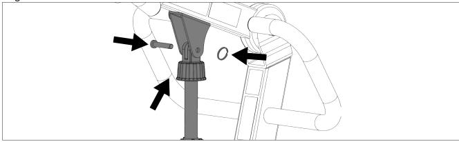
**Step 9**: Attach the footplate to the base using the two hooks by lowering it onto the top surface of the base. Make sure the hooks are sitting in between the two small blocks protruding at the back of the base.
