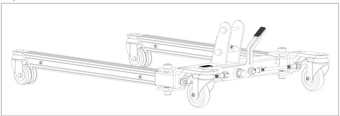
Step 2: Remove all the plastic caps, then all the bolts, nuts and washers on the base bracket.
