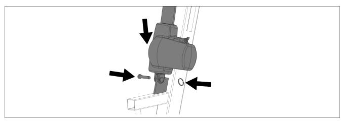
**Step 8**: Secure the upper end of the actuator to the boom bracket using a pin and retaining ring as shown.
