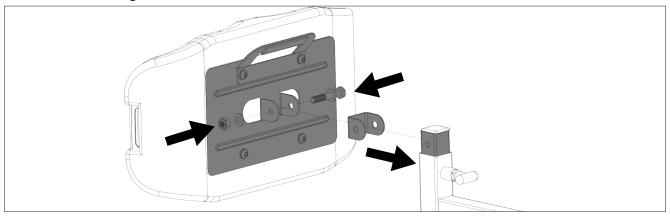
**Step 11**: Insert the kneepad frame into the tube located on the mast. Pull the handle below the tube to fully insert the frame, and release the handle to secure the frame in place.
