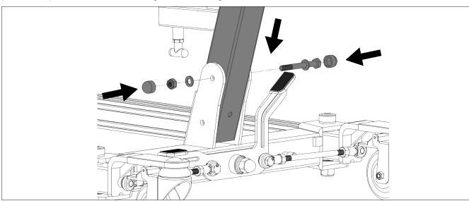
**Step 4**: Other two holes should be aligned, align the holes if needed. Reinsert and tighten the holts using the E7 Tools as follows
