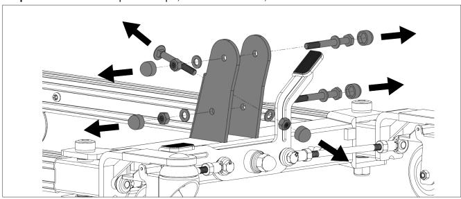
**Step 3**: Insert the mast and align the upper hole on the mast with the upper hole on the bracket. Secure the mast to the bracket using the side bolt and nuts as follows, reinsert the plastic cap after the screw is tightened using the EZ Tools.
