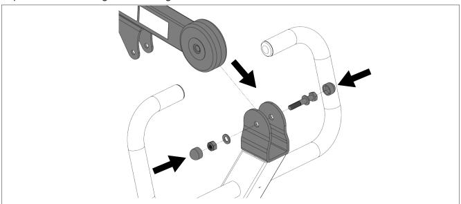
**Step 7**: Secure the lower end of the actuator to the mast bracket using a pin and retaining ring as shown
