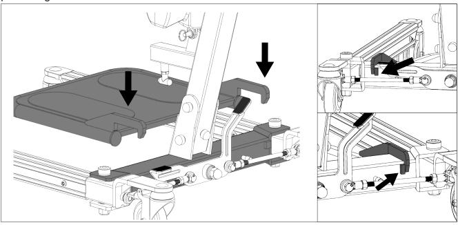
**Step 10**: Attach the included plastic washer to the kneepad frame as shown in the picture below, and place them in between the kneepad bracket. Secure the parts with the bolt, nut and washers using EZ Tools.
