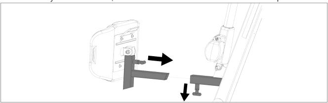
**Step 12**: Use the two handles to adjust the position of the kneepad by sliding it in and out of the tube.
