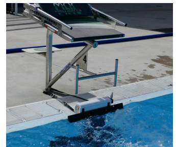
4. Wedge automatically retracts out of the water
