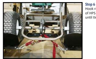
Hook ratchet buckle strap to front of HPS as shown below and tighten until tires are snug to wheel stops.
