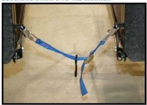
**Step 1**Attach strap with the cam buckle to passenger side of carrier. Open the threaded connector links and attach one each to the tie down loops that are welded to the hinge bracket.
