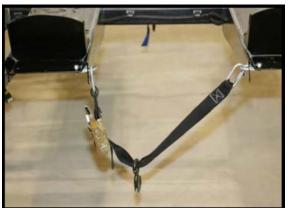
Step 3 Attach strap with ratchet buckle to the tie down loops on the driver side of carrier.
