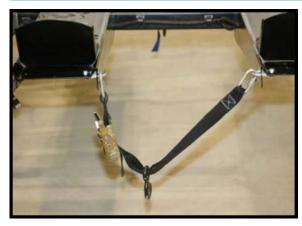
**Step 2**Attach strap with ratchet buckle to the tie down loops on the driver side of carrier.
