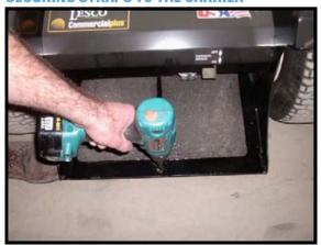
Step 1 Locate center of back edge of sulky deck. Measure in (forward) 3/4" and drill a 1/2" or 5/8" hole on the HPS
