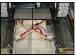
Drive HPS up ramps onto carrier until it hits the wheel stops. Hook cam buckle strap to rear of HPS as shown and pull tight.
