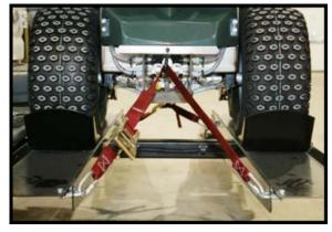
**Step 5**Hook ratchet buckle strap into hole in front bumper of the Magnum.
