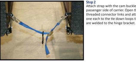
Attach strap with the cam buckle to passenger side of carrier. Open the threaded connector links and attach one each to the tie down loops that
