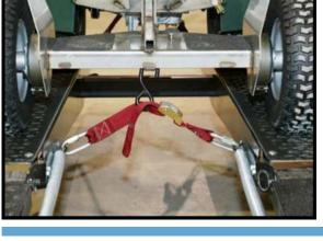
Drive Magnum up ramps onto carrier until it hits the wheel-stop. Hook cam buckle strap to the rear of the Magnum and pull tight.
