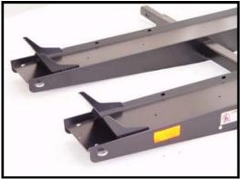
Place wheel stops in position as shown for HPS.
