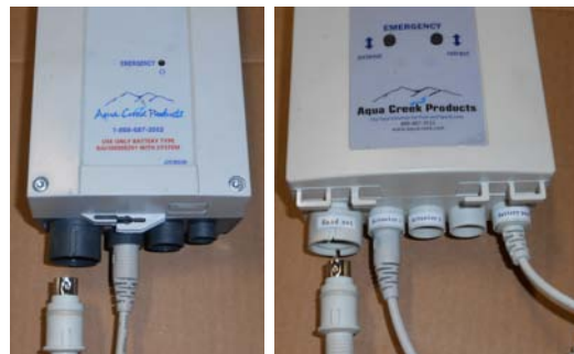
Unplug handset remote from Port A and plug in the known good handset remote
