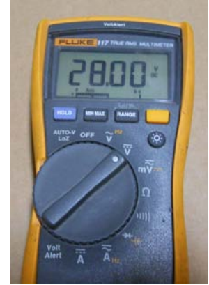
Volt meter should read at least 25.0VDC
