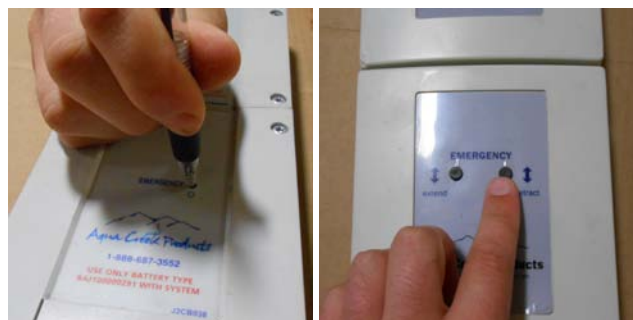
Use a pen to press the emergency Linak button. Use your finger to press the Vito emergency buttons.
