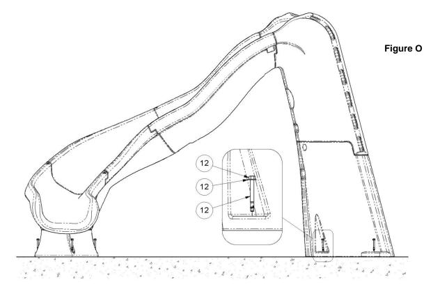
8. Drive the assembled Wedge Anchors (12) through the slide mounting holes until the Wedge Anchor Flat Washers are flush with the slide's surface material, as shown in Figure P.
