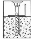
4. Using a power drill and a 1/2" (13 mm) concrete drill bit, drill the holes to a depth of 4" (102 mm). Use tape or a marking on the drill bit to ensure that the hole for the anchor is drilled to the required depth. Maintain drill hole straight and perpendicular for proper holding strength of anchor stud
