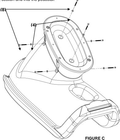
3. Place the assembled runway exit section and pedestal upright so that the pedestal is resting on the ground.
