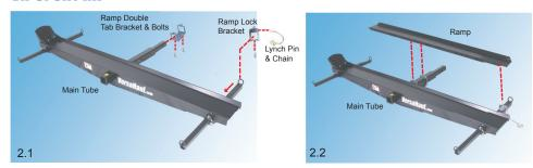
Slide the Ramp Double Tab Bracket over the Main Tube, and secure with the ¼" x ¾" Bolts. Slide the Ramp Lock Bracket over the Tie Down Tube. Do NOT over tighten (Figure 2.1). Slide the Ramp onto the Lock Bracket tabs. Lock the Lynch Pin into place (Figure 2.2).
