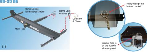
Slide the Ramp Double Tab Bracket over the Main Tube and secure with the ¼" x ¾" Bolts. Slide the Ramp Lock Bracket over the Tie Down Tube. Do NOT over tighten (Figure 1.1). Slide the Ramp onto the Lock Bracket tabs. Lock the Lynch Pin into place (Figure 1.2).
