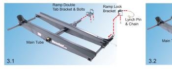
Slide the Ramp Double Tab Bracket over the Main Tube and secure with the ¼" x ¾" Bolts. Slide the Ramp Lock Bracket over the Tie Down Tube. Do NOT over tighten (Figure 3.1). Slide the Ramp onto the Lock Bracket tabs. Lock the Lynch Pin into place (Figure 3.2).
