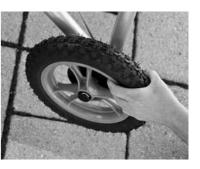
the black button at the centre of the wheel and push the wheel axle into the axle hole. Release the button when the wheel is in its end position. 3. Hold the tire and push/pull the wheel back and forth laterally to check if the wheel is properly secured.
